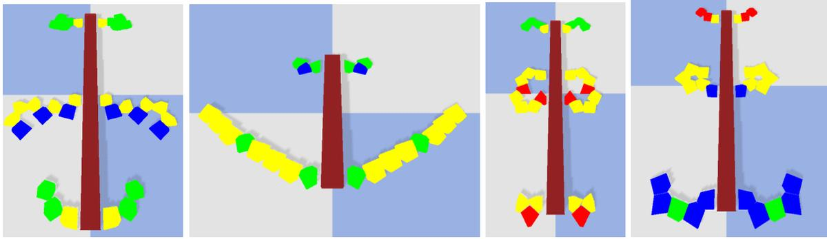
Fig. 3. Morphologies of highest performance (fittest) robots evolved in each environment. **Left:** Hexapod morphology evolved for the high friction, flat surface (environment *A*, table II). **Center-Left:** Quadruped evolved for the low friction, flat surface (environment *B*, table II). **Center-Right:** Hexapod evolved for the high friction, inclined surface (environment *C*, table II). **Right:** Hexapod evolved for the low friction, inclined surface (environment *D*, table II).
