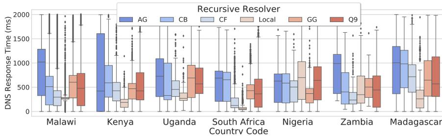
Fig. 3: DNS response time for each DNS recursive resolver across the vantage countries under 4G
