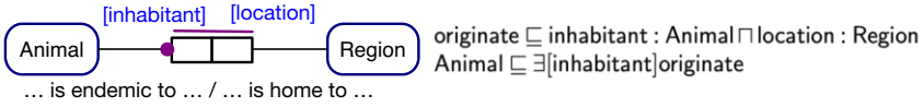
Figure 1. Left: Object-Role Modeling diagram about animals (Q729 in Wikidata) being endemic to a region (Q82794), where “... is endemic to ... / ... is home to ...” is a reading label in both directions, originate could be the name of the relationship or Wikidata’s P183 binary property (not shown in the diagram), and [inhabitant] and [location] are the roles as part of that relationship (respectively possibly Q22947 and Q17334923 in Wikidata). Right: typing of the relationship and mandatory participation of Animal , in \mathcal{DLR} notation. The verb ‘originate’ is a member of the verb class establish-55.5-1 in VerbNet that has thematic roles agent and theme .
