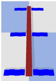
Fig. 1. Pre-designed robot morphology as per related work [6], using material type: *friction*, *restitution* = (0.75, 0.75), indicated by blue legs.
