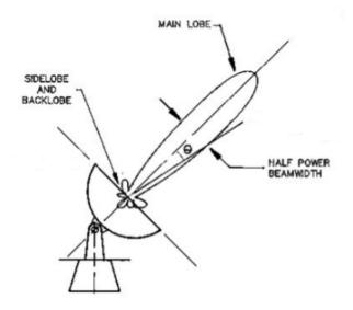
Figure 2.4: Single dish telescope overlayed with the main and side lobes of the receiver pattern. Angular resolution is equal to angle  $\theta$ . Image Source: [70].
