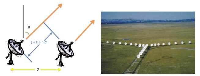
Figure 2.5: A) A single radio interferometry baseline.  $\tau$  is the extra propagation distance and consequently time taken for signal to reach the more distant antenna. B) The Karl G. Jansky Very Large Array (VLA) in North America (http://www.vla.nrao.edu/).
