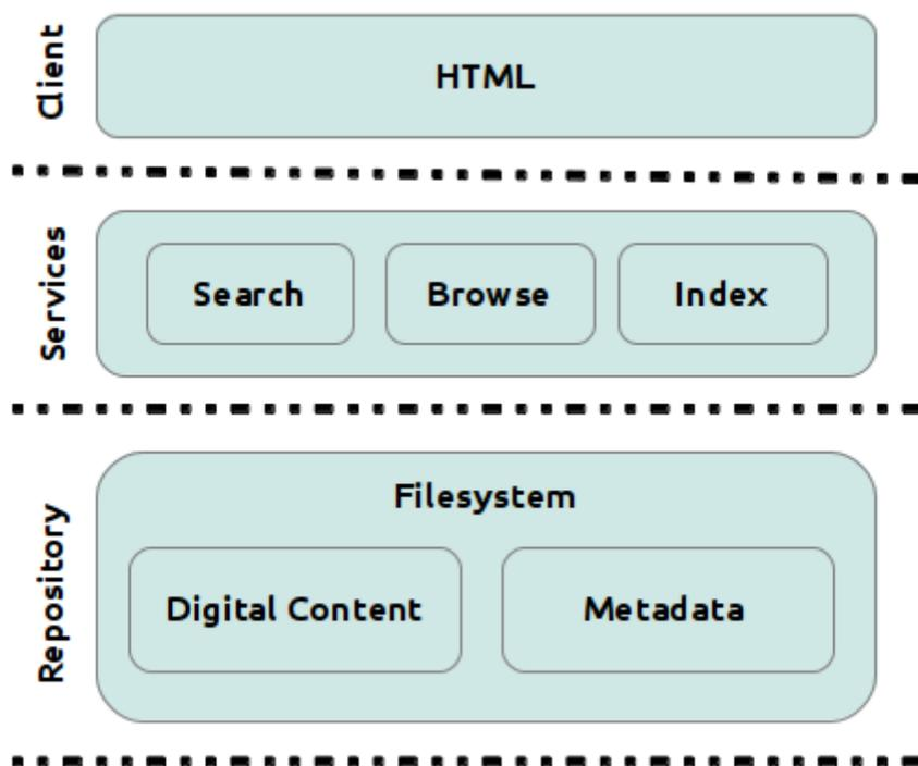
Figure 2. The Digital Bleek and Lloyd System Architecture
