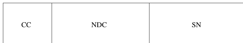
Figure 4: The structure of the GSM MSISDN
